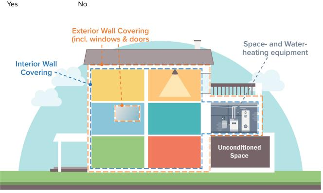
The **building thermal envelope** is the parts of a building (e.g., exterior walls, floors, ceilings, roofs) that enclose conditioned space or provide a boundary between conditioned and unconditioned space. **Conditioned space** is an area or room that is normally heated or cooled by equipment, whereas **unconditioned space** is any enclosed space within a building with no equipment to regulate temperature, like garages or attics.
